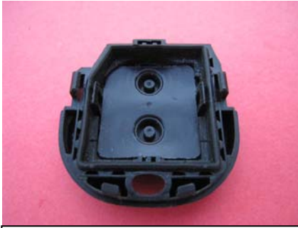
New Silicone Pad should tightly fit in buttons slot.
