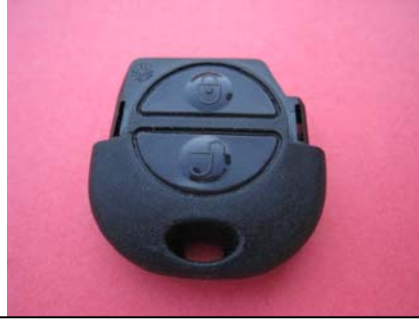
New Silicone Pad should tightly fit in buttons slot.
